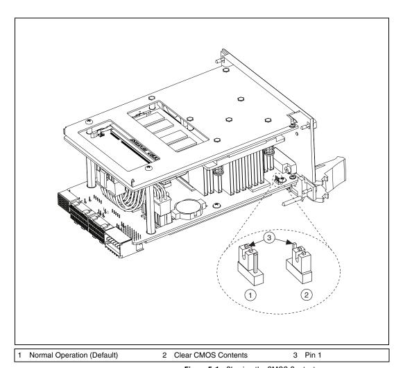
Figure 5-1. Clearing the CMOS Contents
